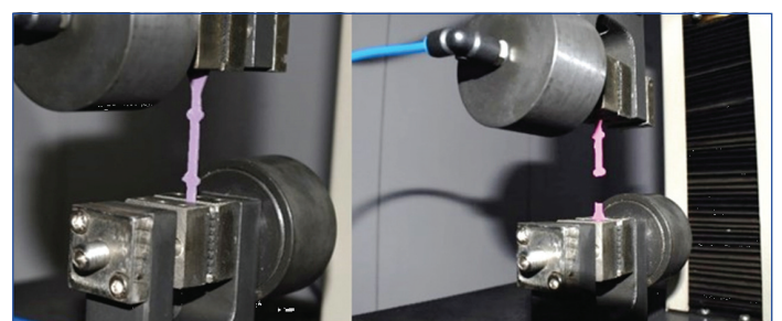
[Table/Fig-5]: The specimen subjected to tensile loading on the UTM.
